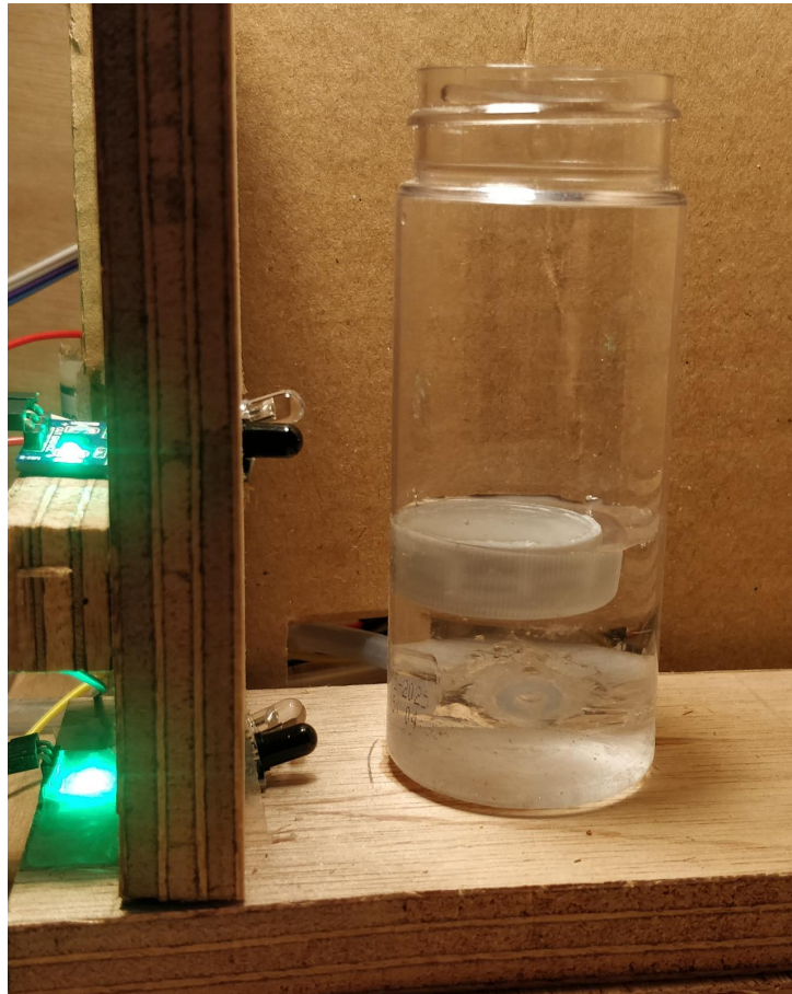
Figure 7.5: Photo of calibration tank with the two IR proximity sensors.
